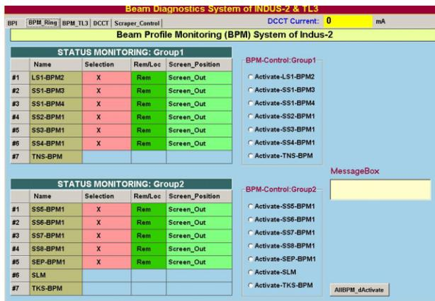
Figure 2: PVSS Panel for BPM control
