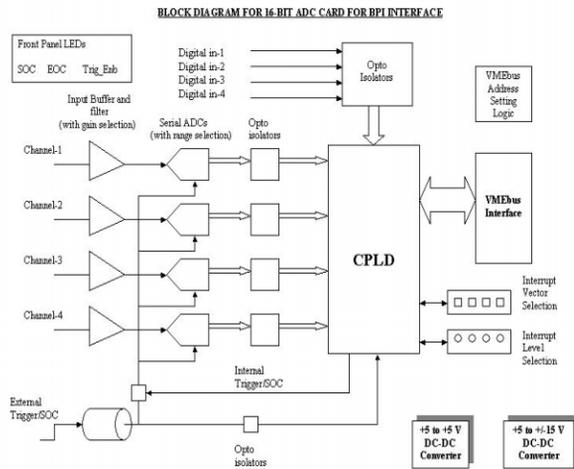
Figure 4: Block Diagram of ADC card
