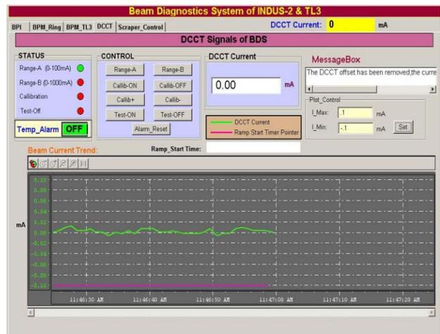
Figure 5: PVSS Panel for DCCT control
