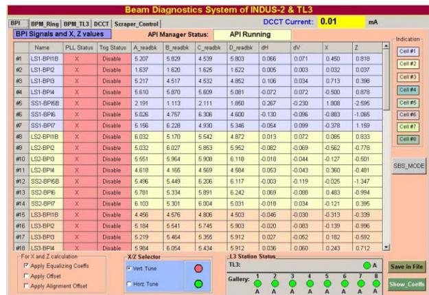
Figure 3: PVSS Panel for BPI control
