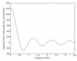
Figure 5: Imaginary part of transverse impedance vs. frequency.
