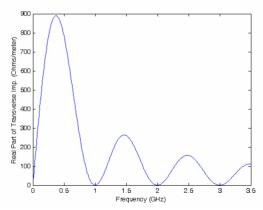
Figure 6: Real part of transverse impedance vs. frequency.
