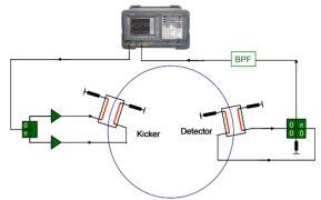
Figure 1: Simplified block diagram for tune measurement.
