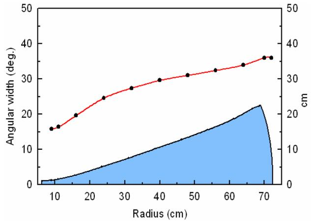
Figure 2: Optimized angular width of the sector as a function of radius and a half model of the hill.
