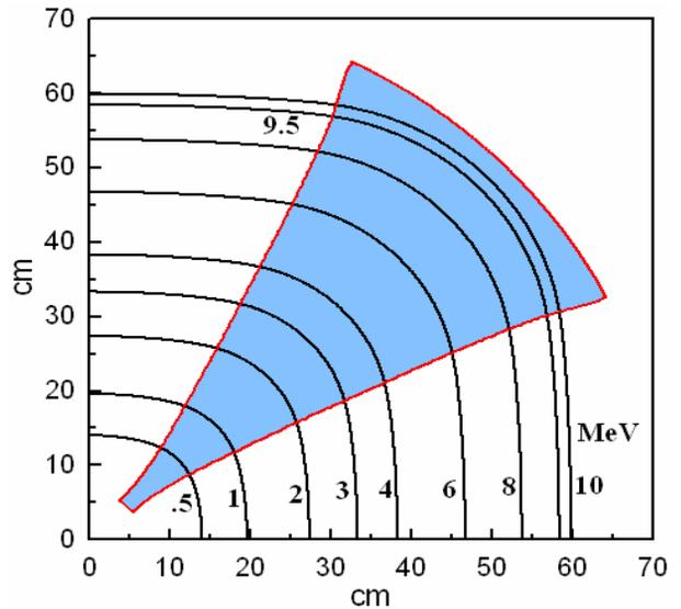
Figure 7: Equilibrium orbits for different energies. The separation between the last two orbits is  $\sim 1.8$  cm.
