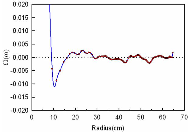
Figure 4: Variation of frequency error  $\Omega(\omega) = (\omega_0 - \omega)/\omega$  as a function of the radius.
