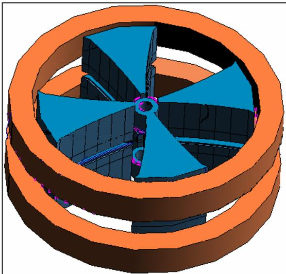
Figure 1: Model of the magnet used for field calculation.
