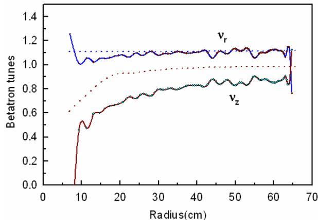
Figure 6: Variation of radial and axial betatron tunes with radius. Dotted curves represent the analytical results.
