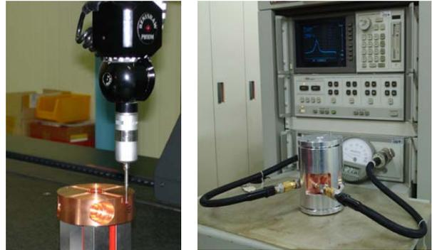
Figure 2(a): A cavity body set up on the 3-D profiler for the dimensional check. b) A cavity BPM assembled in a tightening jig for the microwave measurements before brazing.
