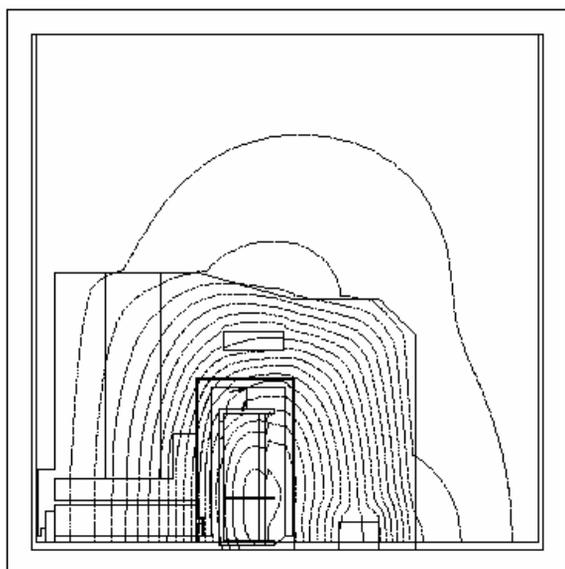
Figure 6: Magnetic lines of forces by ANSYS.
