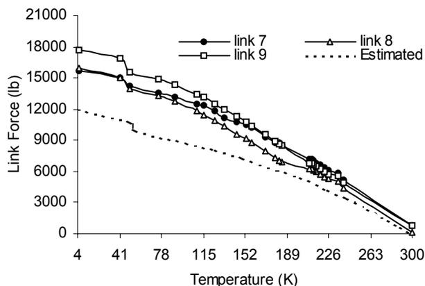
Figure 1: Support link force variation during cool-down of the superconducting coil.
