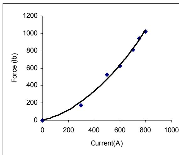
Figure 7: Radial unbalanced force w.r.t. current for 1 mil off-center.
