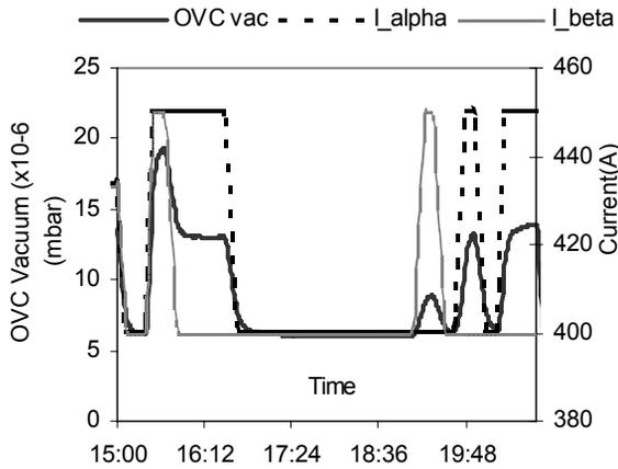
Figure 3: Variation of OVC pressure with alpha and beta coil current.
