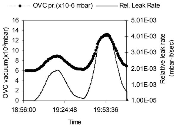
Figure 4: Temporal variation of leak rates and vacuum
