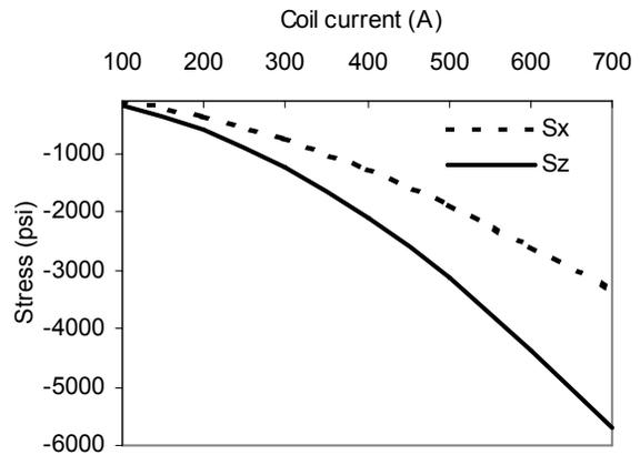
Figure 5: Magnetic stresses on the outer wall of OVC around the median plane at different coil excitations.
