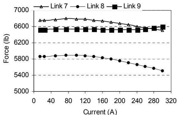
Figure 2: Support link force variation during energization of superconducting coil.
