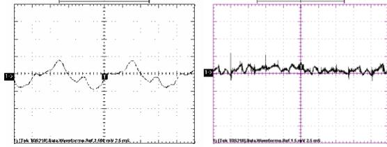
Figure 4. Input Voltage Ripple (left) =  $1V_{p-p}$  and Output Voltage Ripple (right)  $< 5mV_{p-p}$
