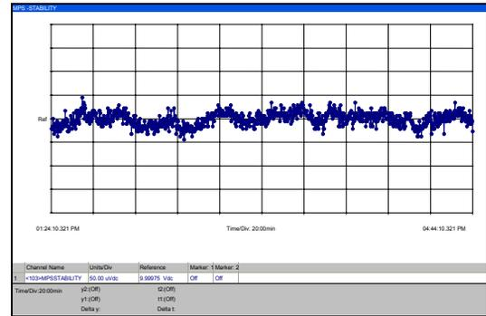
Figure 5. The current Stability Curve (Scale: y-axis: 1div=5ppm; x-axis: 1div=20min)
