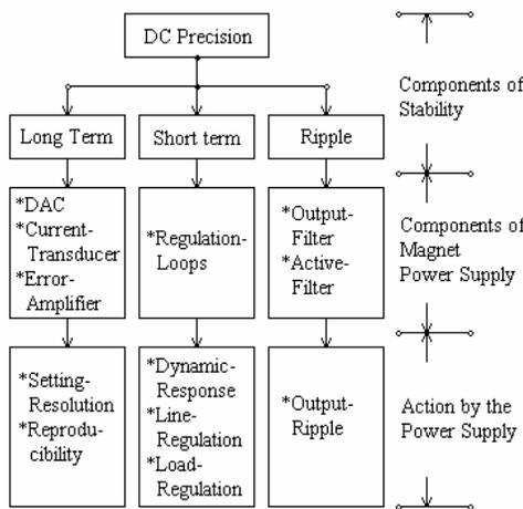
Figure 1: Components of stability of Magnet Power Supply
