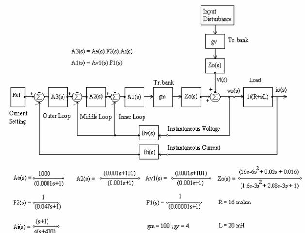
Figure 3 Equivalent model with transfer function
