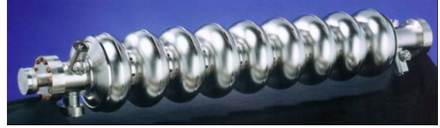
Figure 1: 1.3 GHz 9-cell Niobium cavity of TESLA shape.
