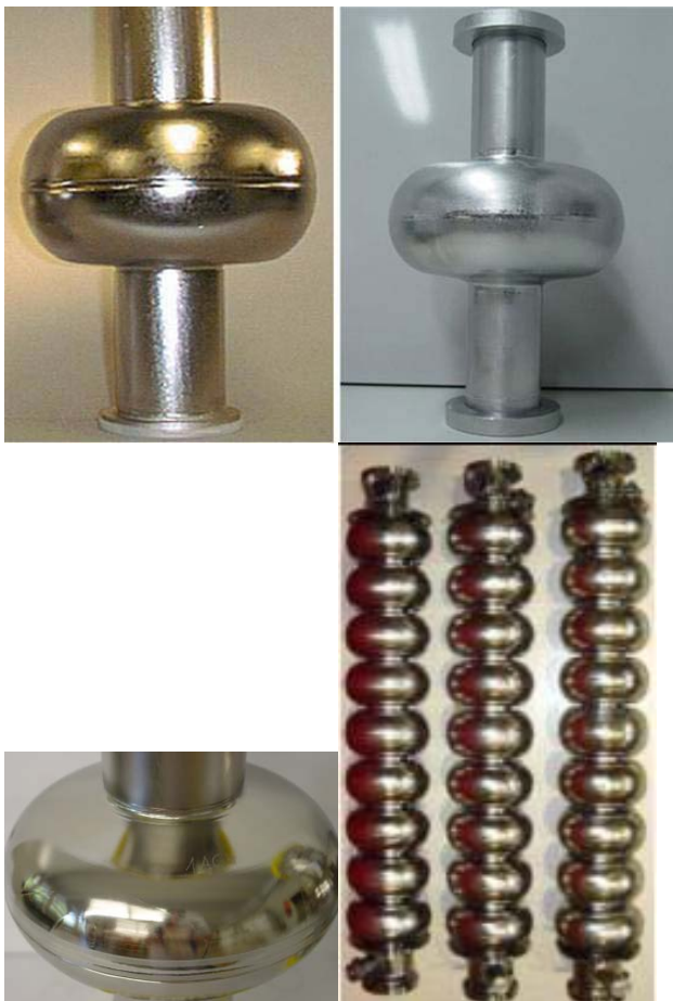
Figure 3: Reentrant (upper left) and Large Grain TESLA (lower left) single cell cavities; Low-Loss single- and nine-cell cavities (left).
