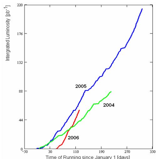
Figure 2: HERA luminosity accumulation 2004-2006
