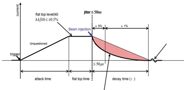
Figure 6: Current waveform of horizontal painting bump
