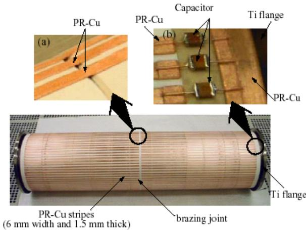
Figure 5: Ceramics chamber of quadrupole
