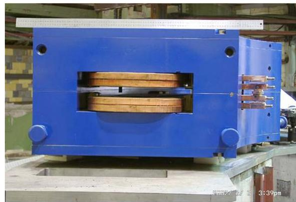
Figure 7: 2.4 T dipole magnet.
