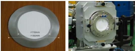
Figure 2: Photograph of exit window coated with P43 phosphor material and its assembly.
