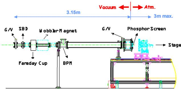
Figure 1: Layout of 50MeV beamline.
