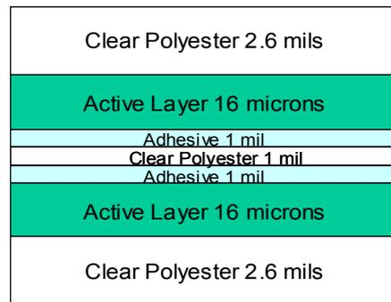
Figure 4: Cross section of Gaf film.
