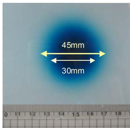
Figure 6: Beam size measured by Gaf film.
