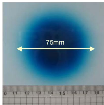
Figure 7: Irradiation uniformity measured using Gaf film.
