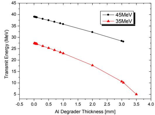
Figure 3: Transmitted proton beam energy vs. Al degrader thickness.
