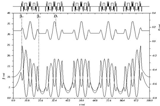
Figure 1: Lattice functions of a SSRF ring super-period.
