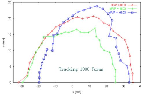
Figure 3: Dynamic aperture tracking in the middle of long straight section.
