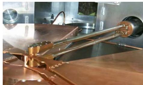
Figure 5 Ion Source installed in the cyclotron
