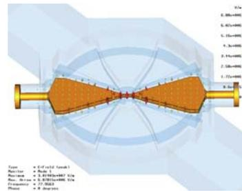
Figure 3 Electric field vector distribution
