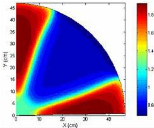
Figure 2 The Measured magnetic field distribution
