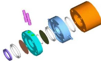
Figure 9 O-18 Water Targetry System
