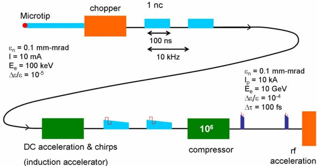
Figure 2: A speculative scheme for producing high-brightness electron beams.
