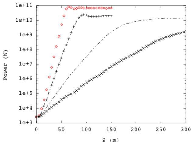
Figure 4: Effect of conditioning on the performance of an FEL. Curve (A) is for unconditioned beams with  $\epsilon_n = 1.2$  mm-mrad, corresponding to the first row in Table 3. Curve (B) shows the improvement of the FEL gain when the beam is conditioned. Curve (C) shows that improvement is more dramatic when the beam conditioning is combined with a stronger focusing,  $\beta_x = 4.4$  m. Finally, curve (D) is for an unconditioned beam but with  $\epsilon_n = 0.1$  mm-mrad [10].
