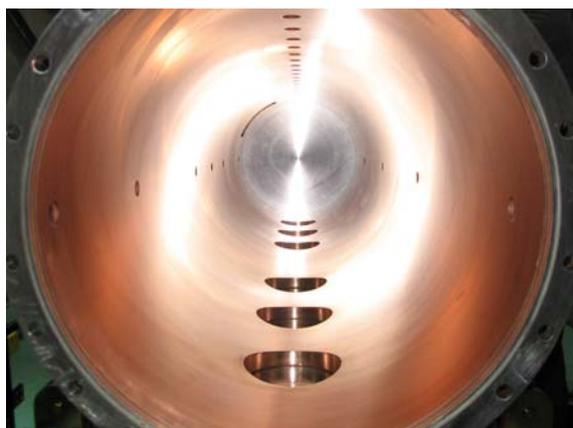
Figure 6: Copper Plated Tank 1
