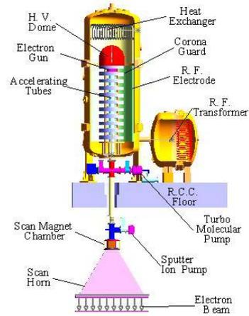
Figure 3: Layout of 3 MeV, 30 kW DC accelerator
