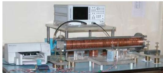
Figure 4: Characterisation of the Linac Cavity
