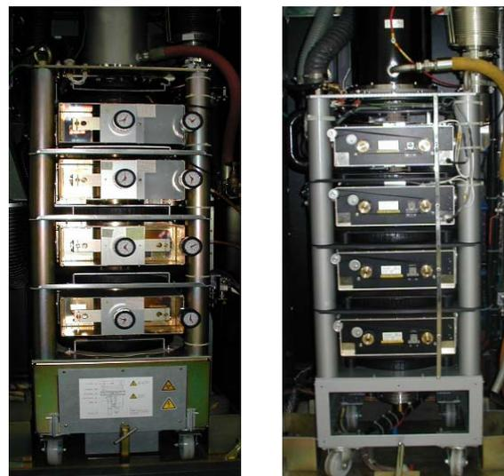
Figure 2: 60kW & 75kW klystron assembly
