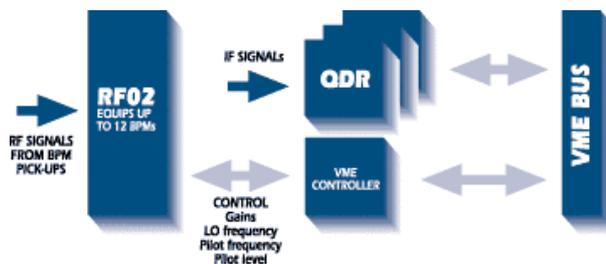
Figure 5: Block diagram of the DBPM2 electronics.
