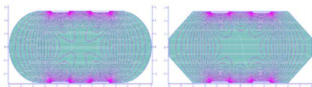
Figure 3: Sensitivities simulation for antechamber BPM and racetrack type BPM, respectively.
