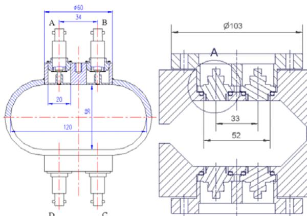
Figure 2: The cross-section of the beam position monitor.
