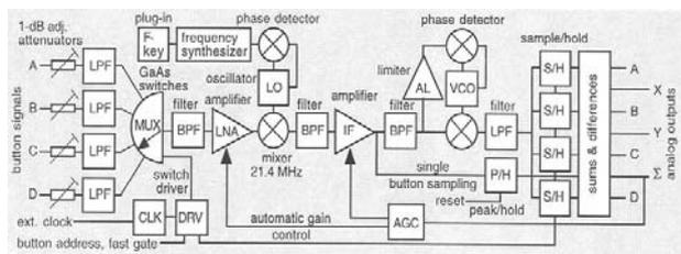
Figure 4: Block diagram of the MX-BPM electronics.
