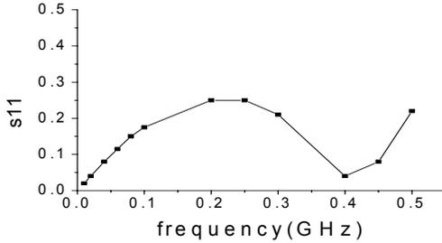
Figure 4: Reflection coefficient vs. frequency
