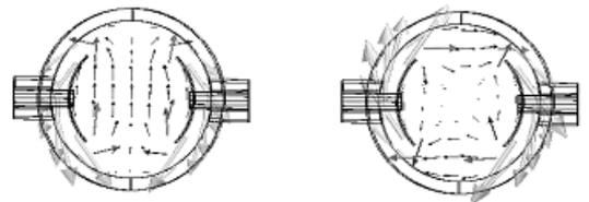
Figure 3.2: B-field distribution on a middle transverse plane in case of even mode (left) and odd mode (right) excitation.
