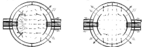
Figure 3.1: E-field distribution on a middle transverse plane in case of even mode (left) and odd mode (right) excitation.
