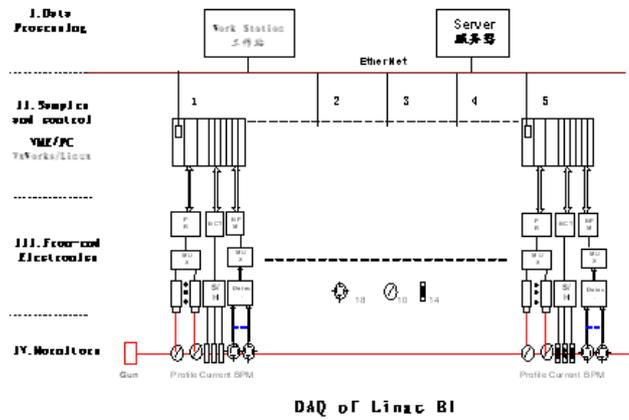
Figure 3: The DAQ structure of linac BI system.
