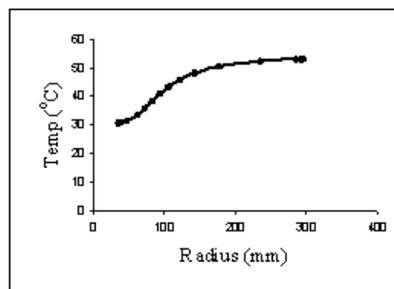
Figure 2: Temperature distribution on the front side of CP for 50 lpm, 22kV case.
