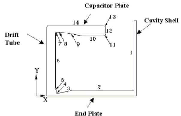
Figure 1: Surface nomenclature of the RF cavity. Y axis shows the electron beam direction and is also the axis of revolution of the RF-structure. X-axis shows the radial direction.
