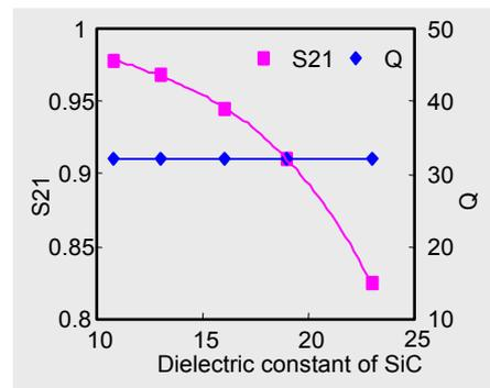
Figure 5: Changes in  $S_{21}$  and loaded Q with dielectric constant of SiC
