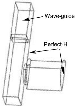
Figure 2: Half-sectioned impedance matching for simulation
