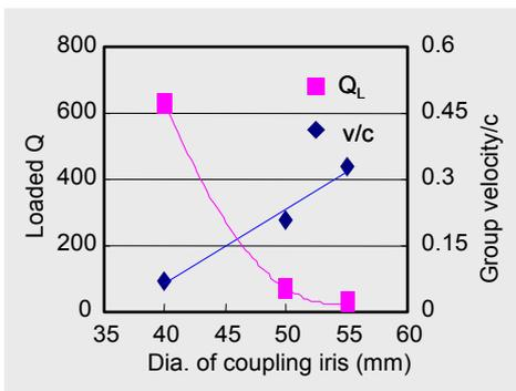
Figure 3: Loaded Q and group velocity with diameter of coupling iris
