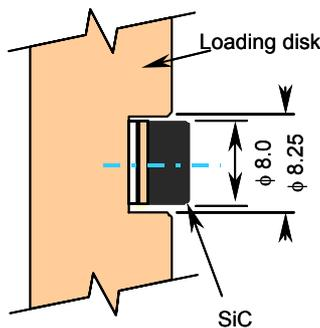
Figure 4: SiC disk brazed on loading disk
