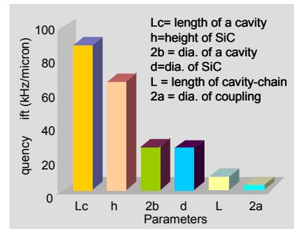
Figure 7: Frequency shift due to the dimension of  $TM_{011}$  mode cavity and SiC disk
