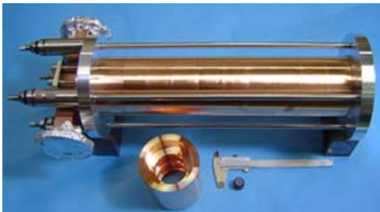
Figure 9: Test model of 50 MW class SiC rf-load
