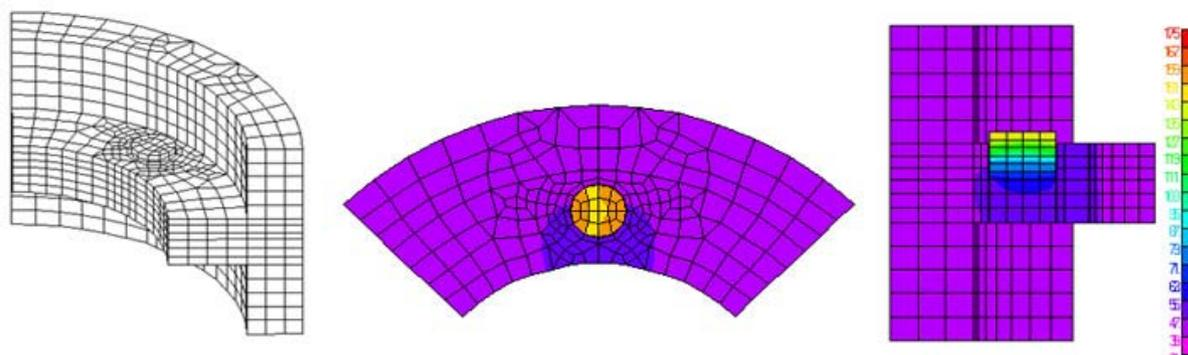
Figure 8: Thermal analysis of the  $TM_{011}$  main body using NASTRAN V70; FEM model and temperature distribution of  $TM_{011}$  cavity and SiC disk
