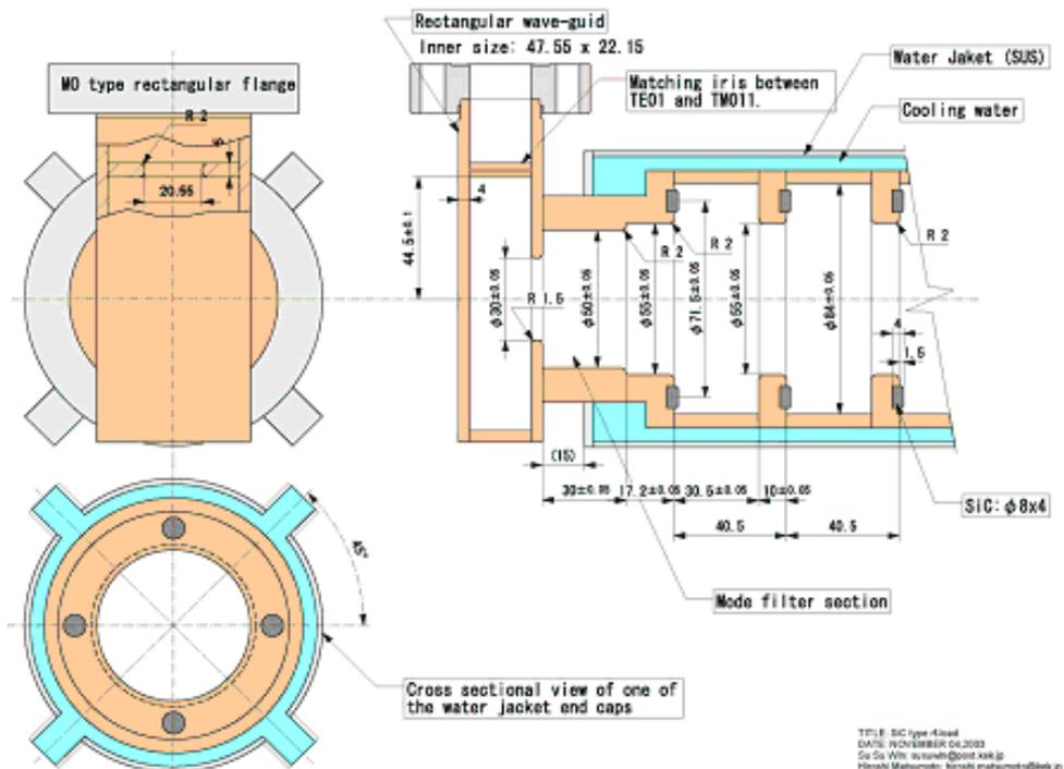
Figure 1: A conceptual drawing of 50-MW Class SiC rf-load
