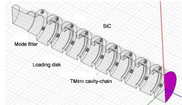
Figure 6:  $TM_{011}$  mode half-cavity chain for the simulation
