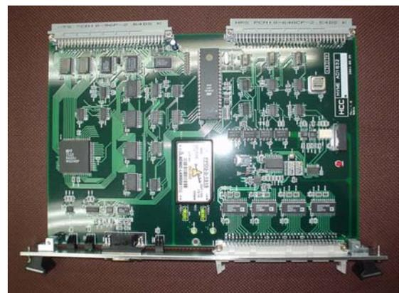
Figure 5: A picture of VMEbus Analog Output Board
