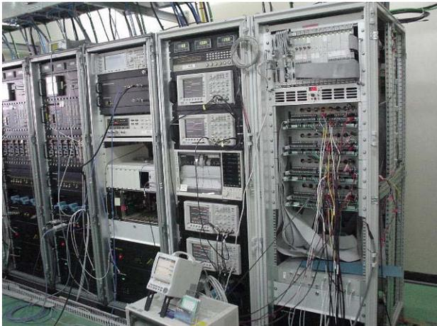
Figure 2: A picture of LLRF & Current RF Control System
