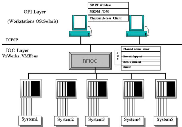
Figure 6: Structure of RFIOC Control Software
