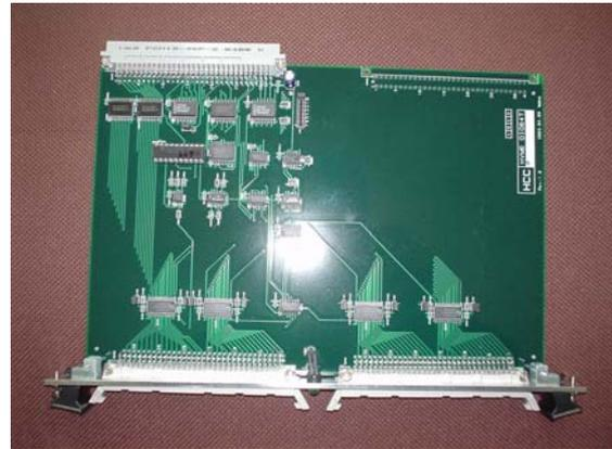
Figure 4: A picture of VMEbus Digital In/Output Board
