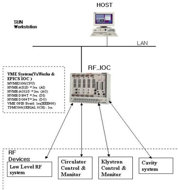
Figure 3: Structure of New RF Control System
