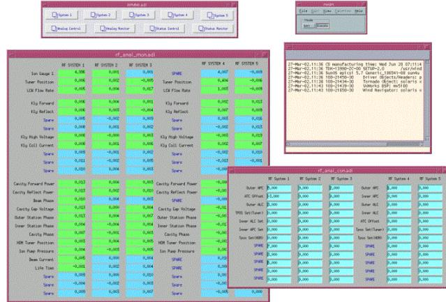
Figure 7: User Interface of RF IOC
