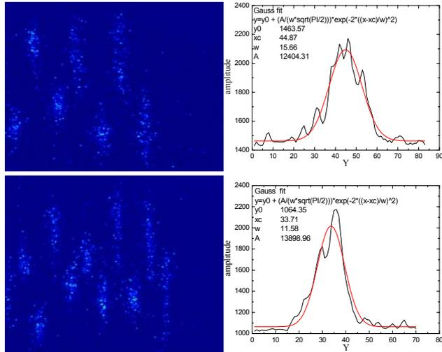
Figure 11: Solenoid effect on bunch size in a bunch train (upper: solenoid off, lower: solenoid on).
