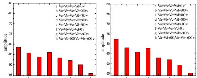
Figure 8: Left and right frequency sidebands amplitude variation in different voltage patterns.
