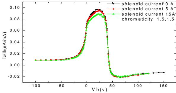
Figure 9: Solenoid effect on EC generation.
