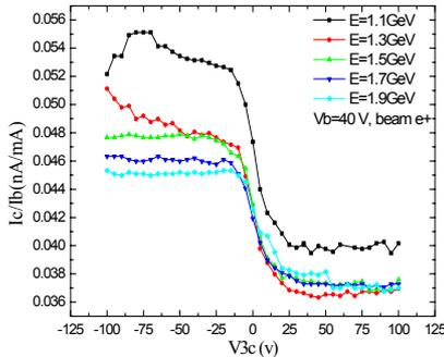
Figure 6: Normalized  $I_c$  changes with  $V_c$  in different energies.
