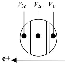
Figure 5: Modified electrode plates in the chamber.
