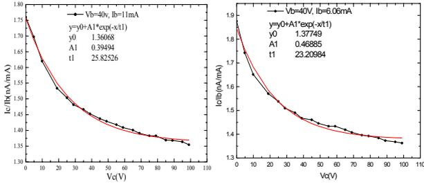
Figure 4: Normalized  $I_c$  as a function of clearing voltage at different bunch current.
