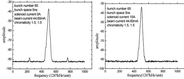
Figure 10: Solenoid effect on sidebands (left: solenoid off, right: solenoid on).
