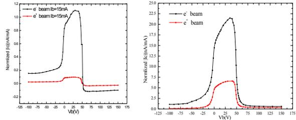
Figure 2: EC current  $I_c$  as a function of the bias voltage  $V_b$  (right: PED1V-U, left: PED4-2V).
