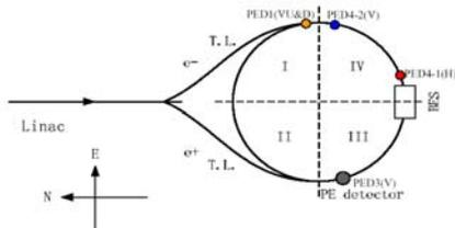
Figure 1: Positions of the 5 EC detectors around the ring.
