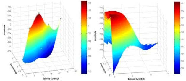
Figure 12: Left sideband variation when chromaticity and solenoid field change (left:  $E=1.3\text{GeV}$ , right:  $E=1.89\text{GeV}$ ).
