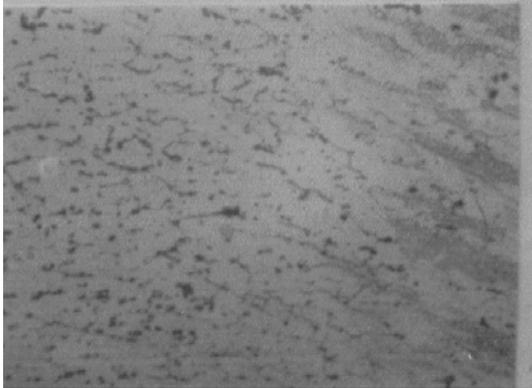
Figure 2: Fusion zone/HAZ/Base metal
