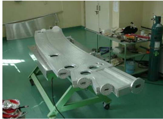
Figure 4: Welded dipole vacuum chamber
