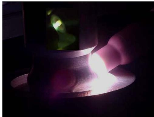
Figure 1: Welding of BPM port
