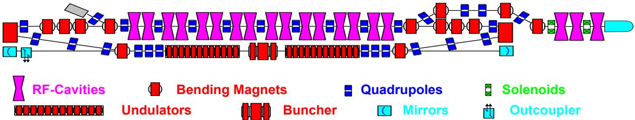
Figure 2: Scheme of the first stage of the Novosibirsk high power FEL.
