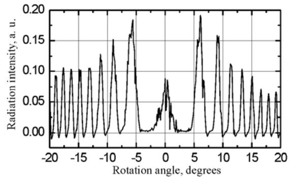
Figure 4: Results of the Fabri-Perot interferometer rotation angle scanning (radiation wavelength is  $136\mu\text{m}$ ).
