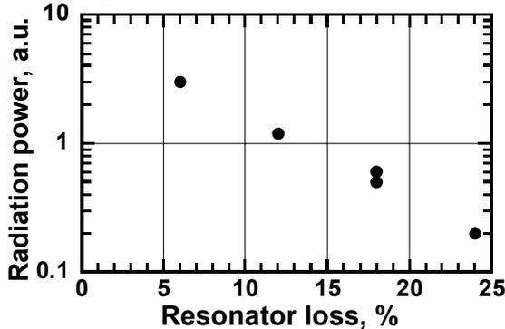
Figure 7: Average intra-cavity power vs. loss per one amplification.
