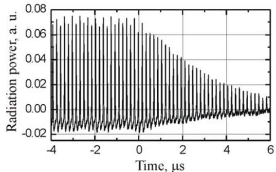
Figure 5: Time dependence of the output radiation power after switching the electron beam off.
