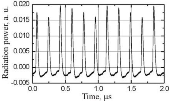
Figure 6: The output radiation time dependence. Electron bunch repetition rate 1.4 MHz is four time less then the optical resonator round-trip frequency 5.6 MHz.
