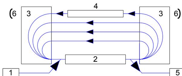
Figure 1: Scheme of the accelerator-recuperator based FEL. 1 - injector, 2 - accelerating RF structure, 3 - 180-degree bends, 4 - undulator, 5 - beam dump, 6 - mirrors of optical resonator.
