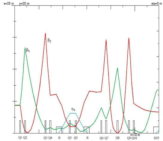
Figure 2. The beam optics of LBT
