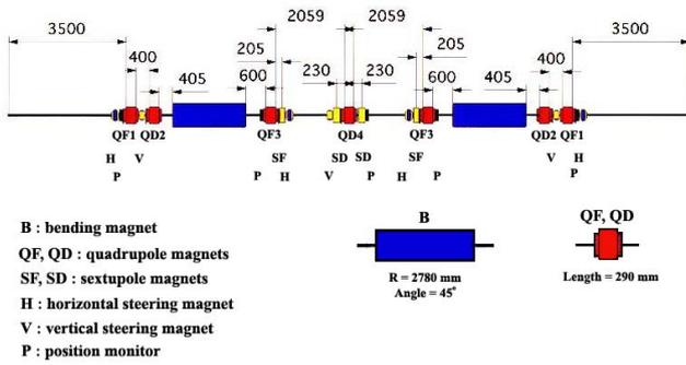
Figure 1. Layout of DBA-lattice (one unit cell) of storage ring
