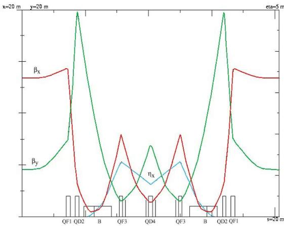
Figure 5. Beam optics of storage ring in a supercell
