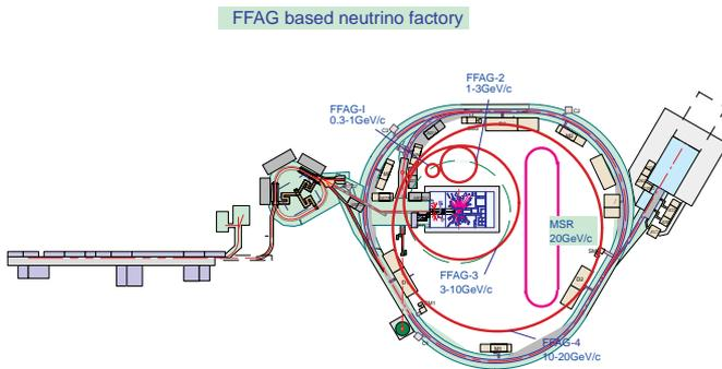
Figure 4: FFAG-based neutrino factory at the Tokai campus
