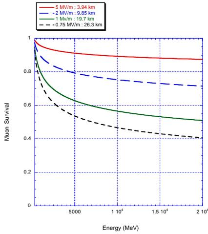
Figure 1: Muon survival rate during acceleration in various accelerating field gradient
