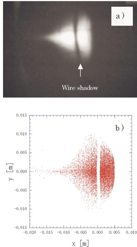
Figure 6: Profile of extracted beam. a): measured, b):tracking simulation
