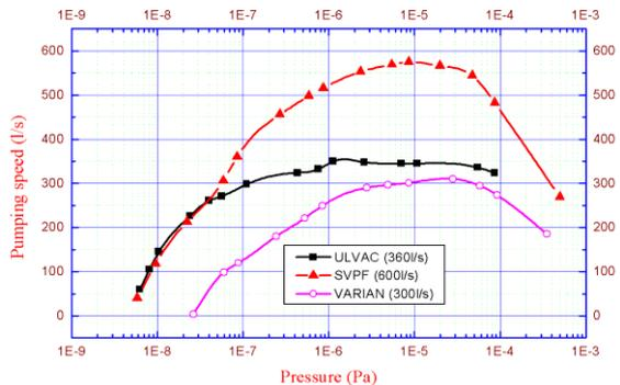
Figure 2: The pumping speed curves of the ion pumps
