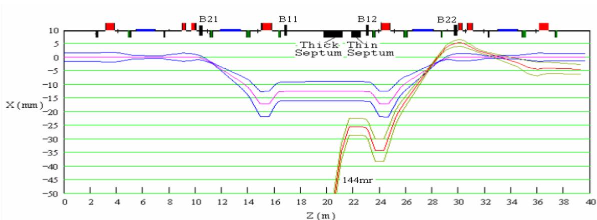
Fig.1 The injection scheme of SSRF storage ring
