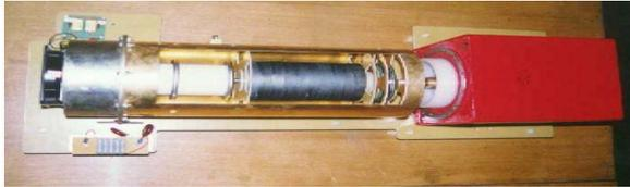
Fig.4 Coaxial structure (a cover removed)
