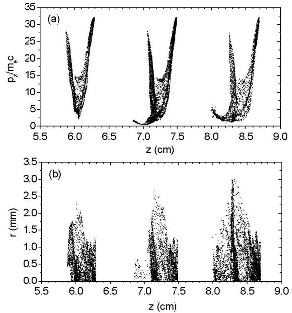
Figure 5: Disruption process of the driver beam. (a) Plot of phase space  $(p_z, z)$  for the driver beam. (b) Plot of phase space  $(r, z)$  for the driver beam.
