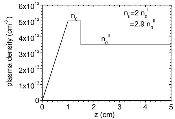
Figure 2: Plasma density profile used for the simulation.
