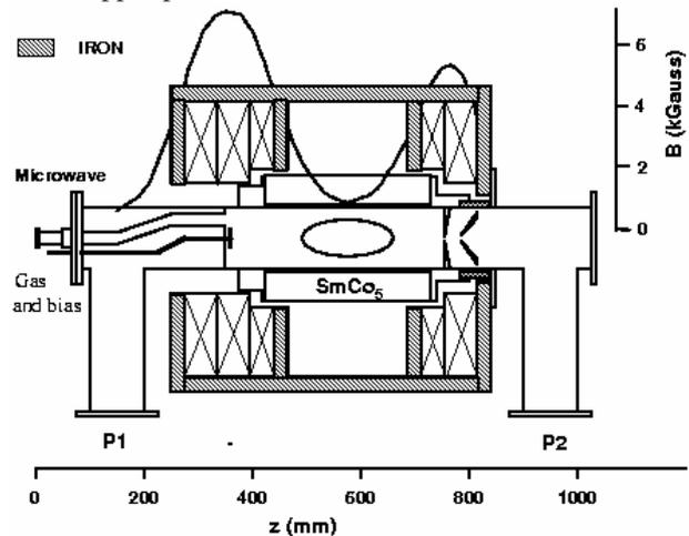
Figure 1: Schematic VEC-ECR
