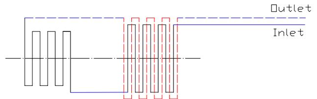
Fig. 6 circulation of cooling liquid helium in the magnet
