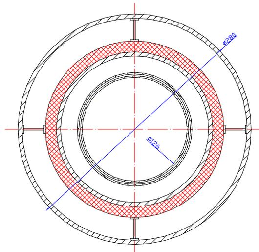
Fig. 5 The cross section of the magnet at SCB
