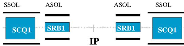
Fig. 1 Superconducting Magnets of BEPB-II Double Rings
