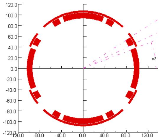
Fig. 2 Cross section of SCQ
