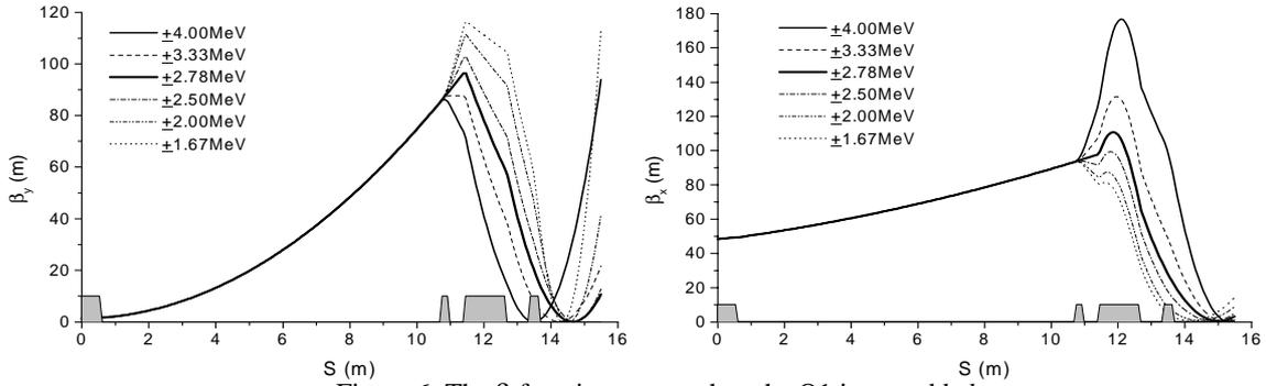
Figure 6: The  $\beta$  function curve when the Q1 is not added
