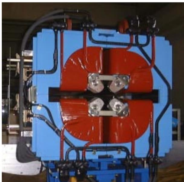
Figure 2: Photographs of the new quadrupole magnet.
