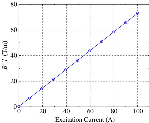
Figure 6: The excitation curve of the integrated field gradient for the sextupole magnet.
