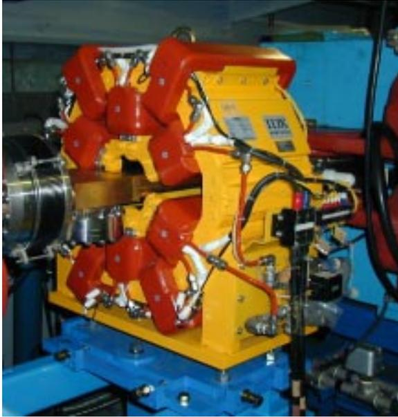
Figure 3: Photographs of the new sextupole magnet installed in the ring.
