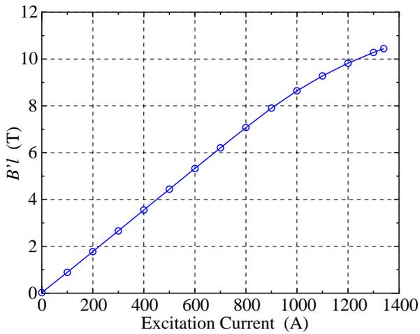
Figure 5: The excitation curve of the integrated field gradient for the quadrupole magnet.
