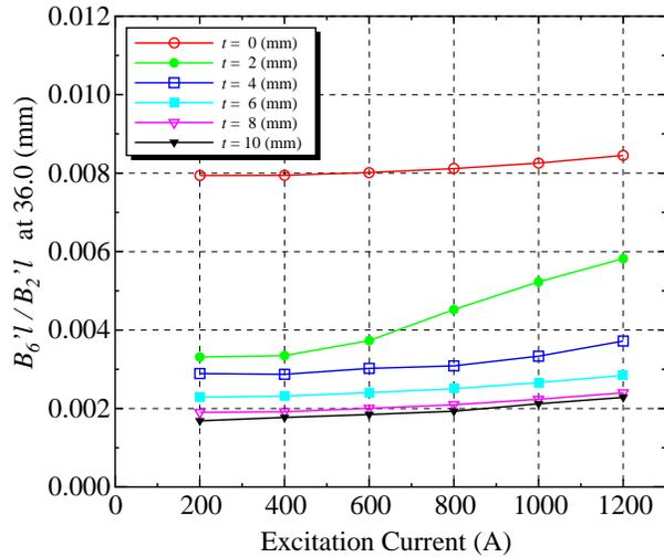
Figure 8: A field gradient ratio of the dominant higher multipole field component (dodecapole field component) to the main field for the quadrupole magnet.
