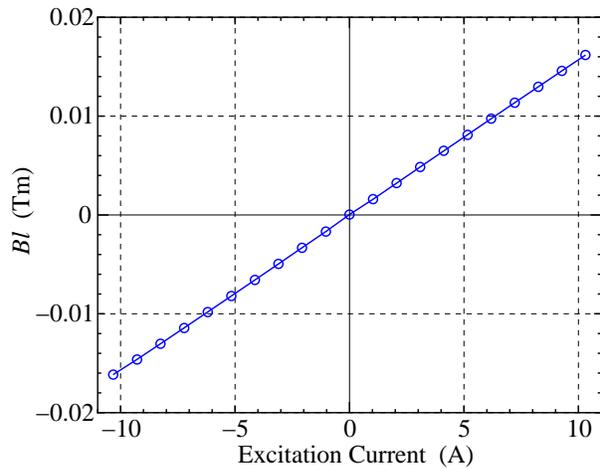
Figure 7: The excitation curve of the integrated field strength for the vertical steering magnet.
