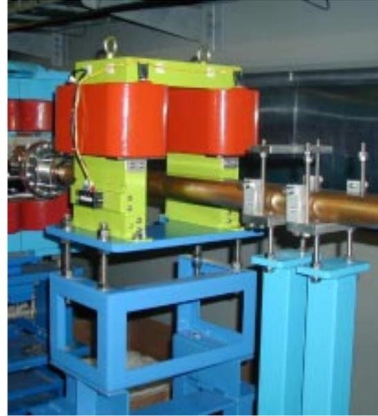
Figure 4: Photographs of the vertical steering magnet installed in the straight section.
