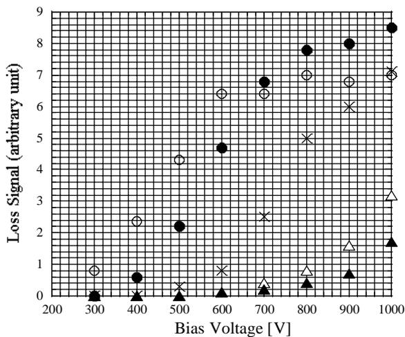
Figure 5: Dependence of the kicker loss signal on the bias voltage of the photo-multiplier
