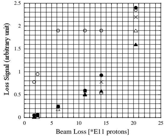
Figure 6: Dependence of the kicker loss signal on the beam loss
