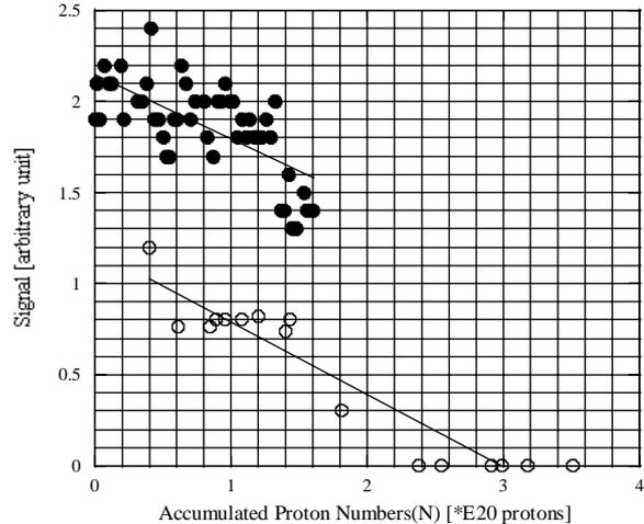
Figure 9: Deterioration of M3 using a scintillation-fiber (Dependence of loss signal due to Bump orbit on accumulated extracted proton numbers)
