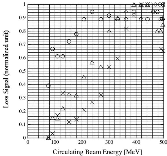
Figure7: Dependence of the loss signal on the circulating beam energy
