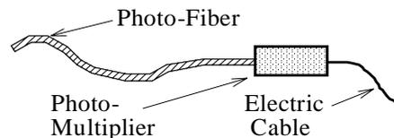
Figure 3: Whole appearance of the loss monitor
