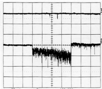
Figure 8: Beam loss during H<sup>-</sup> injection (40MeV)
