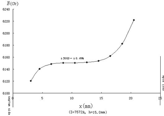
Fig. 6 The distribution curve of the main field
