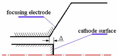
Fig.5. Relative position of focusing electrode and cathode
