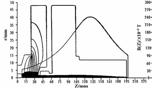
Fig.3. Electron trajectories in the electron gun at the focusing electrode ( $\phi_1=16.8\text{mm}$ )
