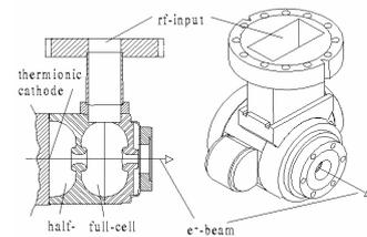
Figure 2: Cross section and 3D-view of the rf-gun [6].
