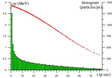
Figure 3: Momentum-time phase space distribution at the rf-gun exit with histogram.
