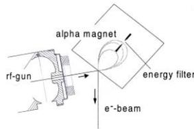
Figure 6: rf-gun and  $\alpha$ -magnet layout.
