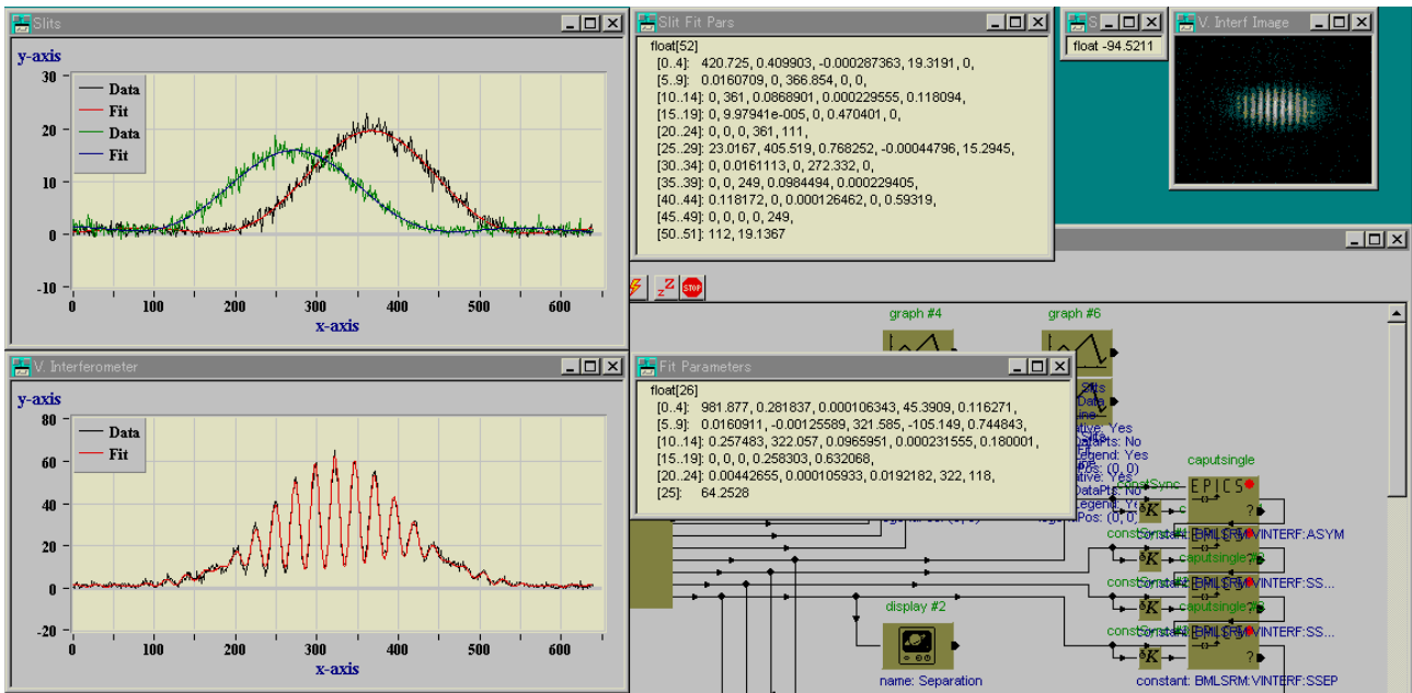
Figure 8: SR monitor data acquisition and analysis system. The curves in the upper left are the single-slit components of the interferogram measured with a shutter, and the lower curve is the resulting 2-slit interferogram. The separation and unequal heights of the single-slit peaks are the result of mirror distortions due to heating, and have to be corrected for to measure the beam size accurately.
