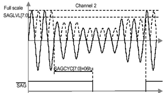
Fig.2. the generation of SAG signal
