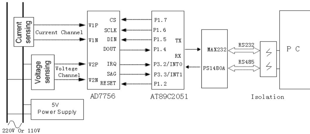
Fig.1 Hardware structure of the system
