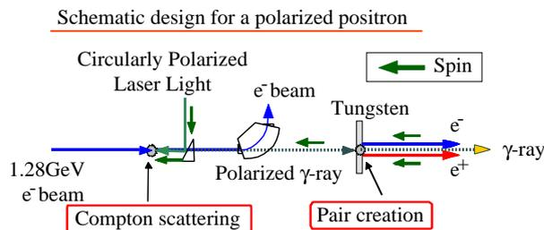
Figure 1: Schematic illustration of a polarized positron generation
