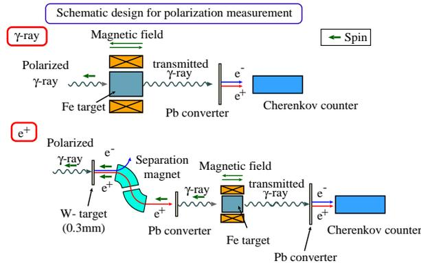
Figure 4: Schematic view for polarization measurement
