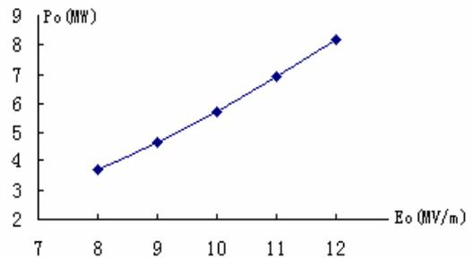
Fig.5. Input power for different accelerating field
