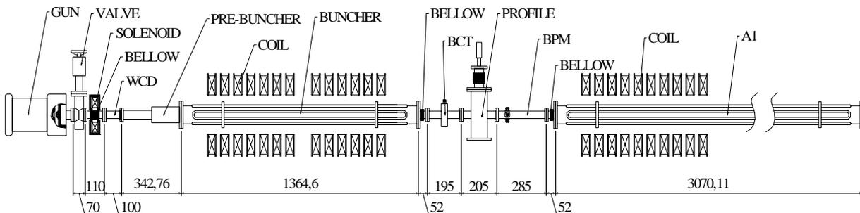
Fig.1. Pre-injector of the SSRF linac
