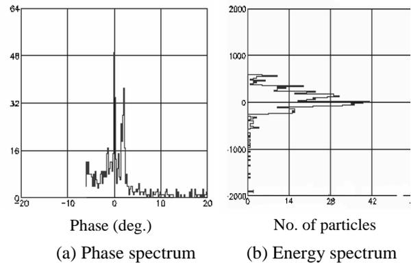
Fig.3. Characteristics of the bunch for 2.0nC at the exit of the buncher. In (a), the vertical axis is the number of the particles, and in (b), the vertical axis is the energy spread of the particles with respect to the center-particle
