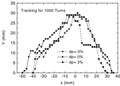
Figure 3 Dynamic aperture in the middle of long straight for the dispersion-distributed hybrid mode
