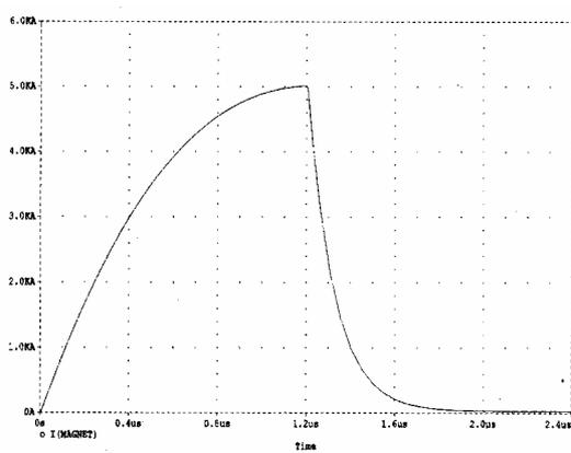
Fig 1 The injection kicker pulse for Indus-1
