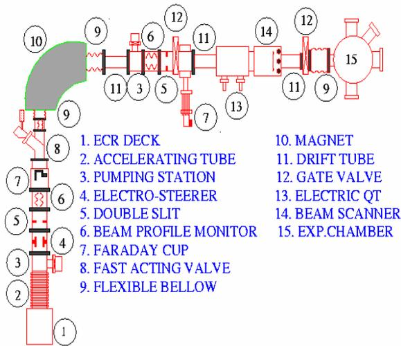
Figure 2: Schematic of the low energy ion beam facility
