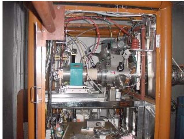
Figure 1: ECR source, extraction system, vacuum pumps, gas bottles, UHF transmitter on high voltage platform.
