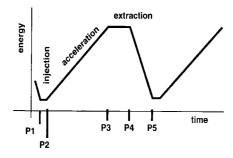
Figure 2: Typical machine cycle of 50-GeV main ring. P1-P2(injcection):0.12s, P2-P3(acceleration):1.9s, P3-P4(extraction):0.7s, P4-P5:0.7s, total:3.42s. Slow extraction of 50-GeV, duty factor:0.20, average current: $15.6\mu$ A.
