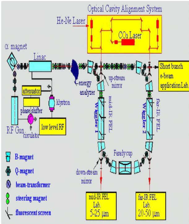
Fig. 1 Schematic Diagram of BFEL
