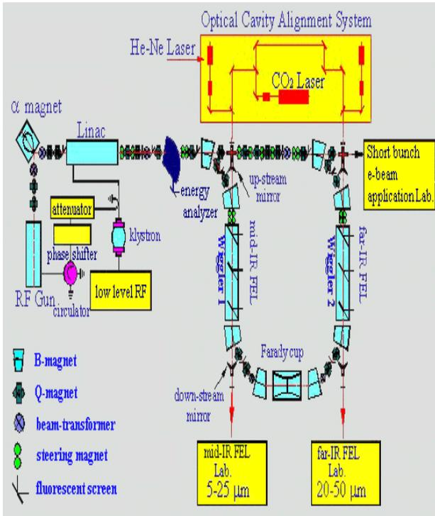
Fig. 1 Schematic Diagram of BFEL
