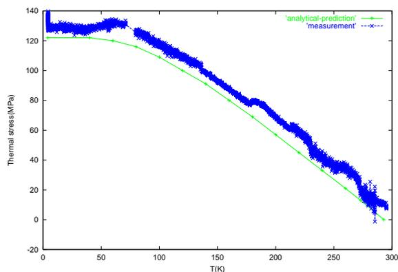
Figure 12: Stress at outside Cu coating surface
