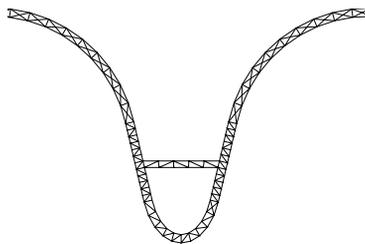
Figure 2: Actual stiffening system using Nb welded rings
