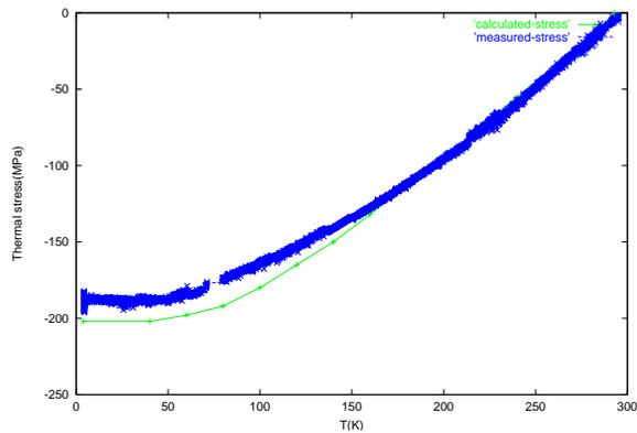
Figure 11: Stress at inner Nb surface
